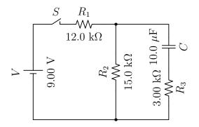
(a) Label the currents  $I_1$ ,  $I_2$ , and  $I_3$  from left to right with each current moving up in its vertical wire. In the steady state,  $I_3 = 0$  (otherwise Q would be changing, which would not be "steady state"). Applying the Kirchhoff's junction rule to the top junction.
